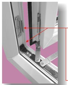
Fit Stay Guard Elite approx 75mm centres from the internal corner as show here. Secure using 4.8 X 25 carbon steel zinc coated screws GT STAY-GUARD ELITE is a simple, easy and effective method of enhancing security for windows.
